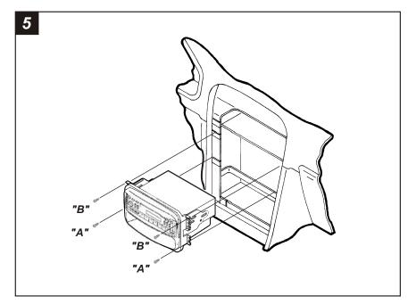
Re-connect the battery terminal and test the unit for proper operation. Mount the head unit/kit assembly to the sub-dash with (2) Phillips screws previously removed in step #1 ("A") and (2) #10 x ¾" Phillips Pan-head Screws supplied ("B").
